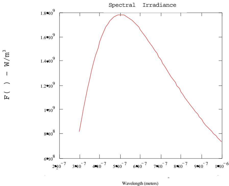
Figure 5: Earth Reflected Solar Light Flux at L2
